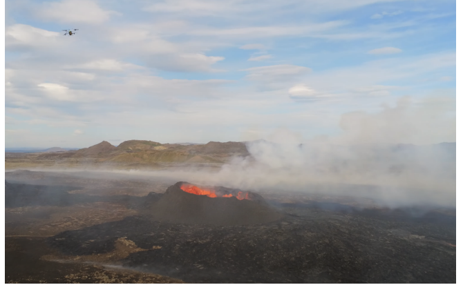
Fig. 1: A UNM VolCAN Dragonfly drone flying into the plume of the actively erupting Litli-Hrtur volcano in Iceland. This expedition involved measuring CO 2 concentrations across multiple transects of the plume to build a plume model and estimate the flux of the eruption.
