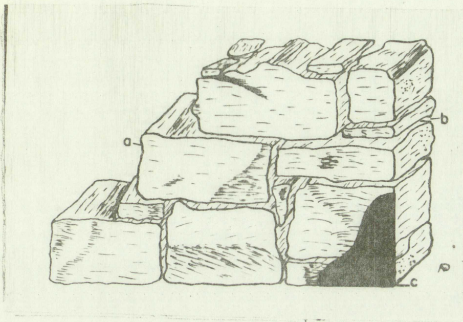
Fig. 10 Sandstone masonry in which the ends of the blocks have been squared: a. sandstone block, b. adobe mortar and c. plaster.
