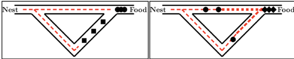
(c) The ants that have taken the short path have arrived earlier at the food source. Therefore, when returning, the probability to take again the short path is higher.
