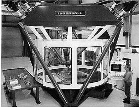
(a) A machine tool based on the Stewart Platform (Ingersoll Rand)<sup>6</sup>
