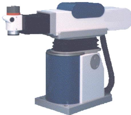
Figure 10 The RT3300 cylindrical robot (Seiko)
