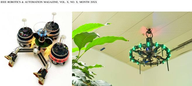
Fig. 1. The swarmanoid robots. (a) Three foot-bots are assembled around a hand-bot and are ready for collective transport. The hand-bot has no autonomous mobility on the ground, and must be carried by foot-bots to the location where it can climb and grasp interesting objects. (b) An eye-bot attached to the ceiling has a bird's-eye view of the environment and can thus retrieve relevant information about the environment and communicate it to robots on the ground.
