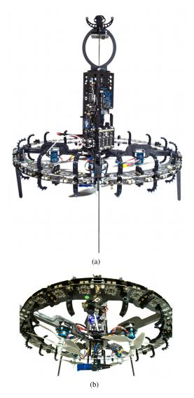
Fig. 5. The eye-bot platform. (a) The ceiling attachment system and the  $24 \times 6.5 \times 6.5$  cm rectangular structure housing the batteries and main PCBs. (b) The four contra-rotating coaxial rotors, the circular 3D range and bearing communication system, and the pan-tilt camera with the laser pointer.
