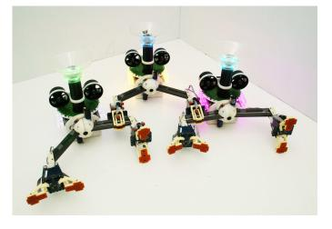
Fig. 4. Three hand-bots assembled together. The hand-bot is an autonomous robot capable of climbing vertical structures and manipulating objects. The grasping hands enable basic manipulation abilities, as well as the possibility to physically connect to other hand-bots forming large structures.
