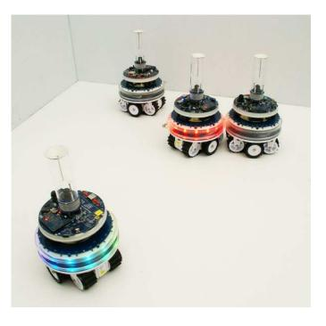
Fig. 3. The foot-bot robotic platform. The foot-bot has a differential drive system that uses a combination of tracks and wheels to provide mobility on rough terrain. Two of the foot-bots in this figure have illuminated their LED communication ring. These RGB coloured signals are detectable by the onboard cameras of other foot-bots.
