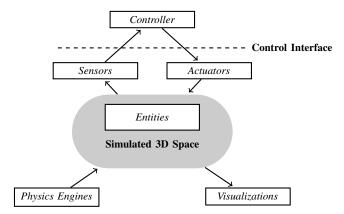
Fig. 6. The architecture of the ARGoS simulator.
