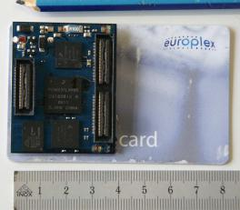
Fig. 2. The half credit card size i.MX31 main processor board.
