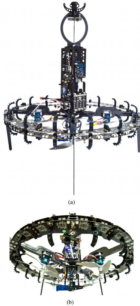
Fig. 5. The eye-bot platform. (a) The ceiling attachment system and the  $24 \times 6.5 \times 6.5$  cm rectangular structure housing the batteries and main PCBs. (b) The four contra-rotating coaxial rotors, the circular 3D range and bearing communication system, and the pan-tilt camera with the laser pointer.
