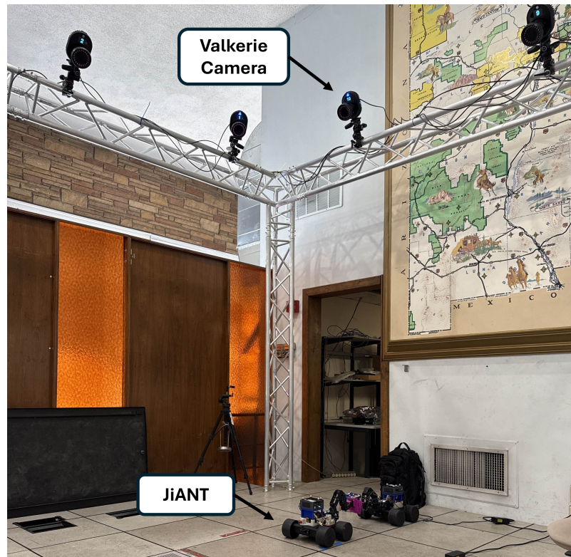
Figure 2.5: A photo of the adopted Vicon camera system workspace and two JiANT robots. In the scaffolding are four Valkerie cameras. The Vicon system comprised of sixteen of these cameras. The pose estimation produced by the Vicon tracking software is transmitted over the same ROS2 network that connects the JiANT robots.
