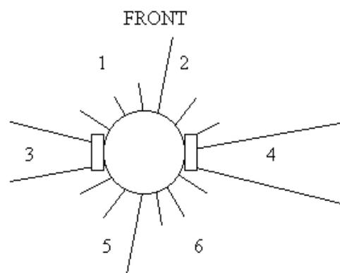
Figure 1: Sonar Sensor Arrangement for Madcat
